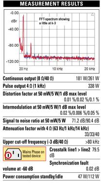
LAB COMMENT: Flawless performance in the lab, superior channel equality and crosstalk attenuation, very broad band, powerful. Low attenuation factor due to the circuitry.
