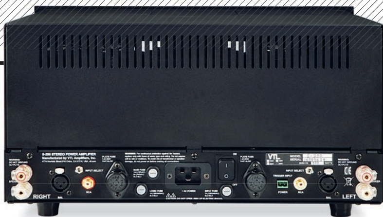
ABOVE: Rear connections include balanced inputs – a selector switch grounds the unused phase for unbalanced. A trigger input allows remote power-up from standby
