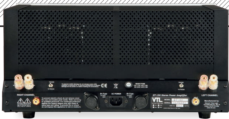
ABOVE: While the push-pull 6550C-based output stage can be switched between tetrode and triode operation [see boxout p25], the speaker outputs are single-tapped
